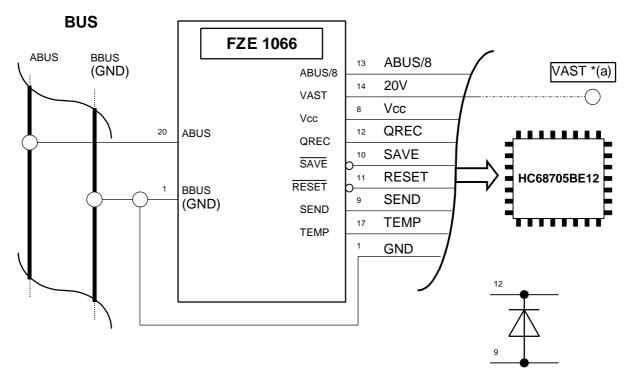
$^{\star}$ (a) If an application is connected, Pin 14 ( $V_{VAST}$ ) serves for voltage supply of this application
